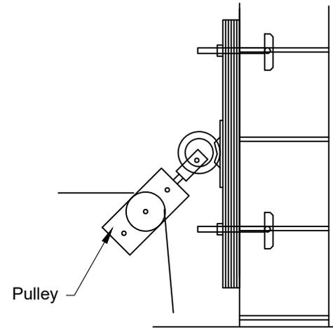
NO. 777 PORTABLE ELECTRIC WINCH OPERATOR ( # REQ'D )
