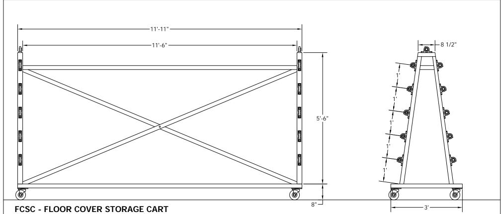
CONSTRUCTED OF STANDARD 3" CHANNEL, ALL-WELDED & SHIPPED AS A COMPLETE UNIT. FLOOR COVERS ROLL ONTO 2" Ø PIPE DRUMS WITH A FULLY WELDED 1" Ø COLD ROLLED STEEL SHAFT AT THE DRUM END. SHAFTS ARE THEN ATTACHED TO FOOT-MOUNTED PILLOWBLOCKS. DRUM OPERATION IS BY REMOVABLE STEEL HANDLE OR OPTIONAL PORTABLE RIGHT-ANGLE DRIVE DRILL.
